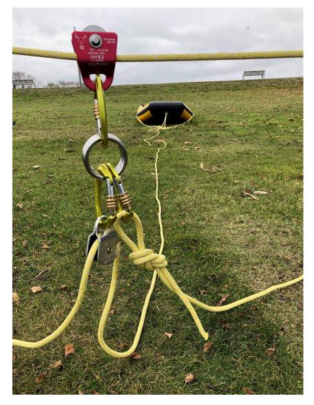
Figure 7: Boat on highline dry rigging using TEC REEP.
