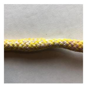
Figure 9: Abrasion on TEC REEP
