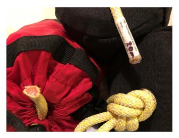
Figure 3: Throw bags retrofitted with TEC REEP. Note red inner core (unsealed).
