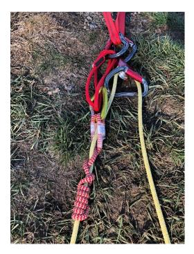
*Figure 2.* Valdotain Truss VT Prusik on TEC REEP low angle system, being changed over with optional karabiner below pulley across both ropes to assist with Prusik minding during haul. In this photo the 80cm Tendon Timber Prusik was used, however the author recommends using the 100 or 120cm variant instead to remove the additional off-set prusik sling as illustrated.
