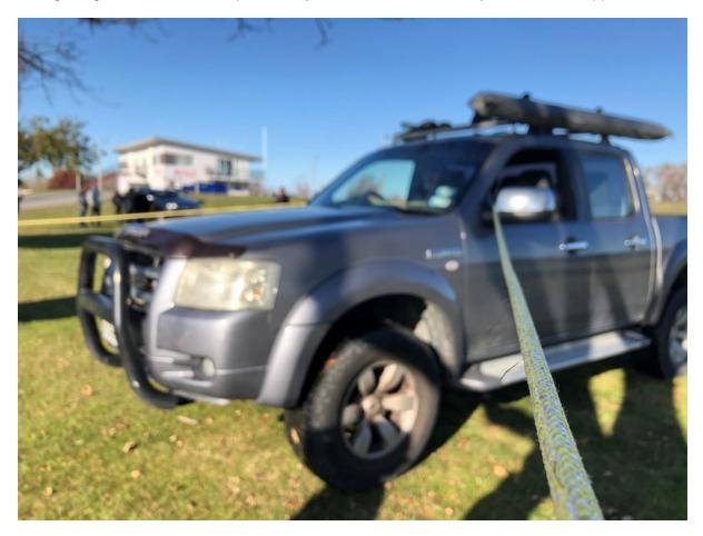
Figure 8: TEC REEP being used for shore based vehicle stabilisation (dry rigging).
