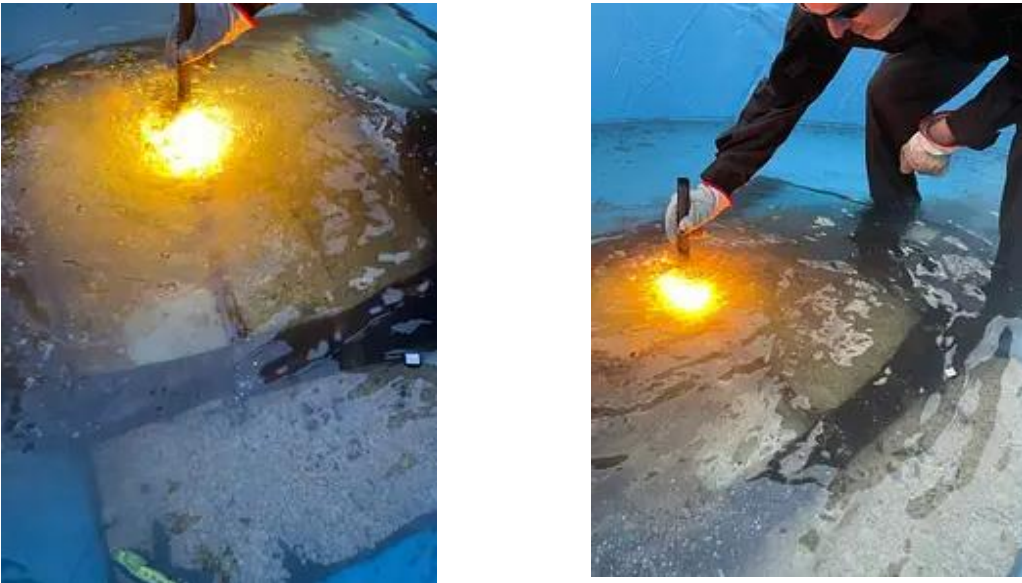
Figure 3. BreachPen Cut #2 through submerged laminated glass.
