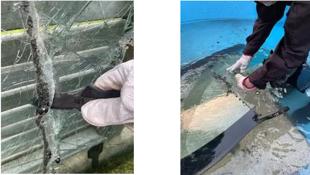
Figure 4. Post-cut cut and lateral separation.
