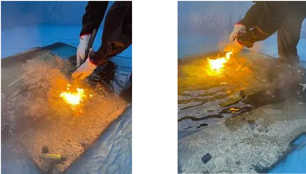
Figure 2. BreachPen Cut #1 through submerged laminated glass.
