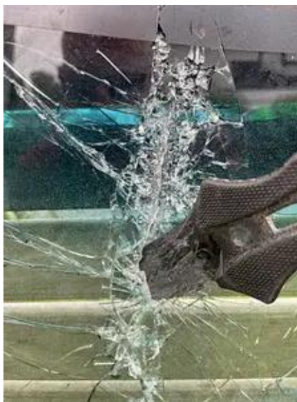
Figure 6. Stitch cutting using serrated knife .
