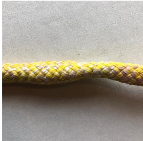
*Figure 10: Flattened TEC REEP by palpation*
