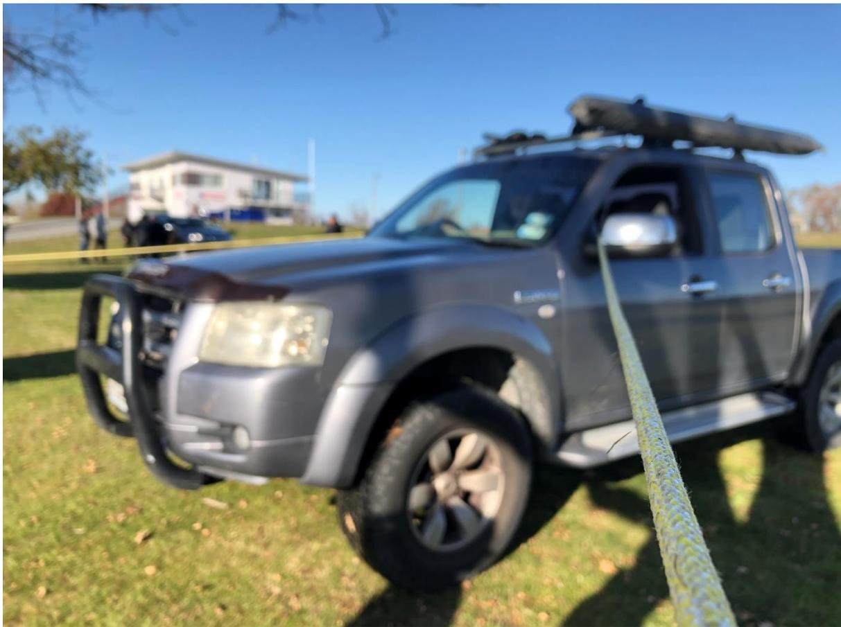
*Figure 8: TEC REEP being used for shore based vehicle stabilisation (dry rigging).*
