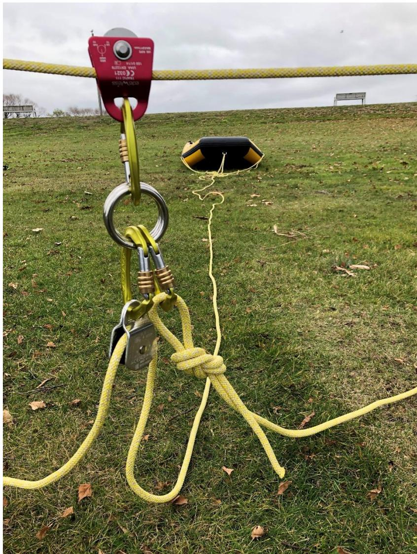
*Figure 7: Boat on highline dry rigging using TEC REEP.*
