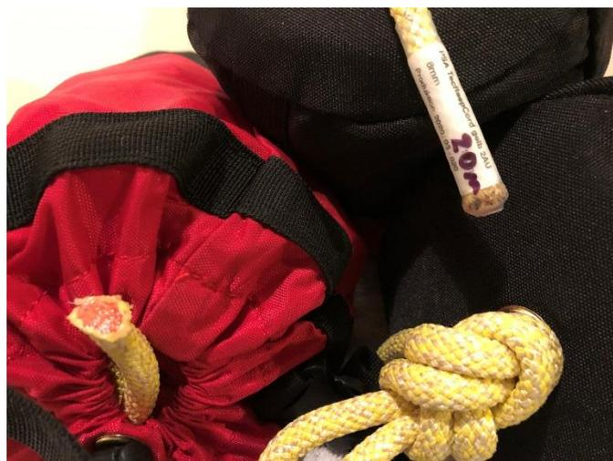
*Figure 3: Throw bags retrofitted with TEC REEP. Note red inner core (unsealed).*
