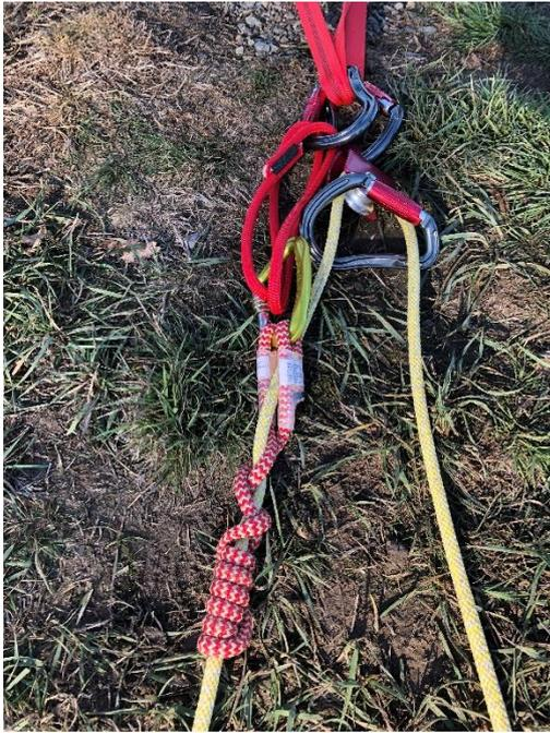
*Figure 2. Valdotaian Truss VT Prusik on TEC REEP low angle system, being changed over with optional karabiner below pulley across both ropes to assist with Prusik minding during haul. In this photo the 80cm Tendon Timber Prusik was used, however the author recommends using the 100 or 120cm variant instead to remove the additional off-set prusik sling as illustrated.*
