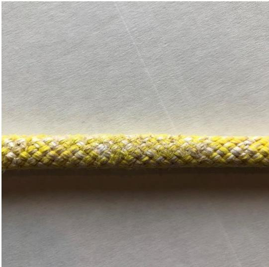
*Figure 9: Abrasion on TEC REEP*
